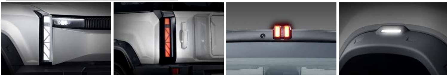
Full LED Prism Headlamp | LED Matrix Vision Rear Lamp | LED J6 High Mount Stop Lamp | Side body Lighted
